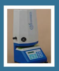
The air permeance of papers has a major importance in the specification of materials for the packaging and printing industries. The air permeance is the flow of air through unit area under unit pressure difference in unit time, under specified test conditions and is expressed in  $\mu$  m/(Pa.s) .
