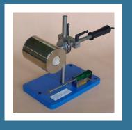
The determination of residue (ash content) on igniniton at  $900^{\circ}$  C is worldwide used to determine the filler content in pulp, paper and board in the routines of Q.C. (Quality Control) of the production lines.
