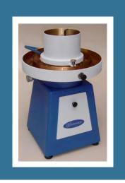
The fiber classificator is used for the separation of pulps into fines, shives and useful fibers fractions.
