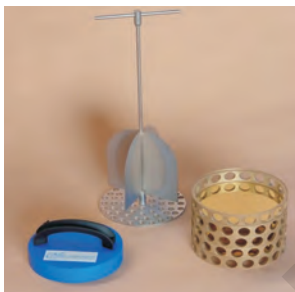
Standard manual mixer, couching weight and drying disc & rings
