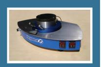
The TD-RK is a laboratory sheet dryer designed to be used along with any Rapid Köthen type Laboratory Sheet Former.
