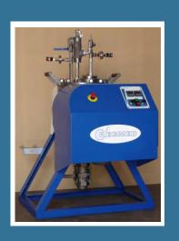
The laboratory reactor model HB-21 has been designed for pilot chemical, semi-chemical and thermal pre-treatments of several types of biomass.
