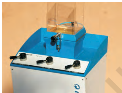
Pneumatic controls for filling, mixing and draining
