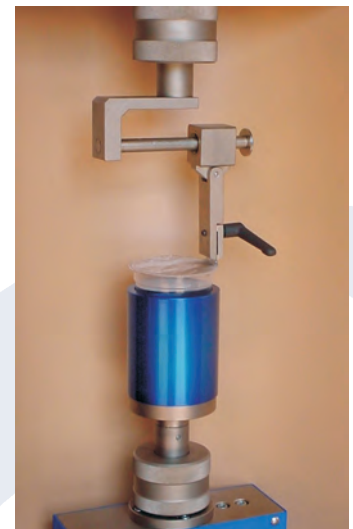
Peel opening force of cups and jars
