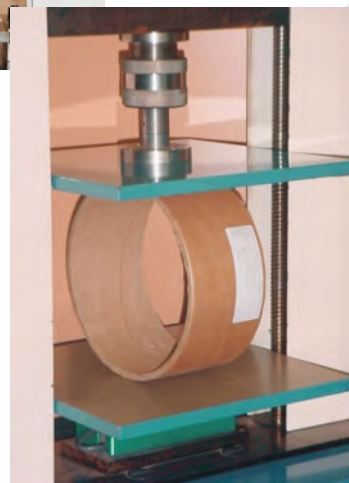
Core compression Applicable standards: ISO 11093-9
