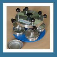
The PVA/4 is designed for preparation of test pieces for the accurate measurement of the WVTR - Water Vapour Transmission Rate - of sheeted materials like paper, board, plastics, aluminum, rubber, etc.
