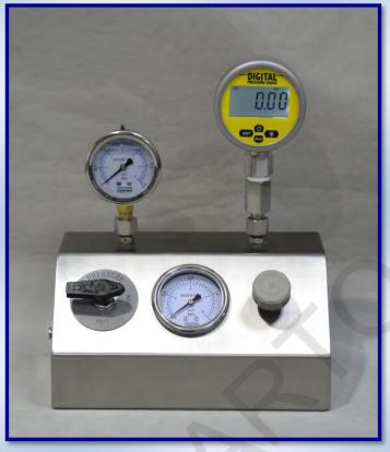
CDP-1 is a device for calibrating the pressure indicator. It allows operator to carry out a visual comparison between the calibrated indicator and the certified one. It is available for analog and digital indicator with different screw thread.
