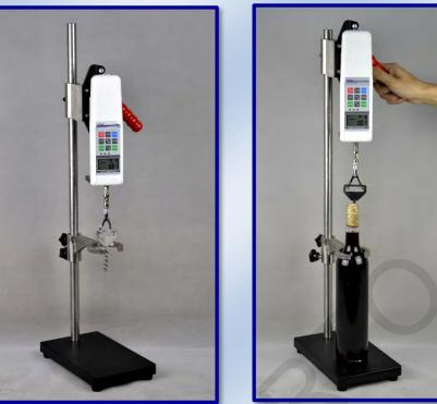
CET-1 Cork Extraction Tester is a force test system. It has been designed for wine producer and cork manufacturing industries. Easy to use, it allows to measure cork extraction or insertion and permits to improve the cork products and assembly/sealing process.
