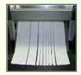
The device is designed as a single sheet cutter. The sample sheet is placed on the metal plate and aligned vertically by means of the knives. When the foot switch is actuated, the sample sheet is grasped, pulled in and the strips are cut. The circular knives and the paper feeder are equipped with a touch protection made of transparent plastic.
