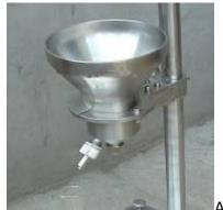
4.1. Adjustable side flow pipe, it can ensure the measure of accuracy and it's convenient for side flow pipe to be checked out again.
