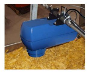
The distance from probe to the surface of the material is from 150mm to 400mm
