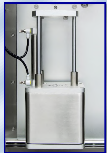
Sample holder with auto angle correction unit
