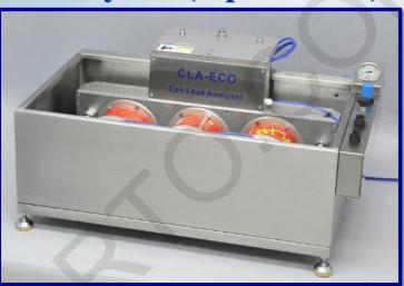
CLA-ECO Can Leak Analyzer is specifically designed for analyzing the secure seal ability of the empty 3-pieces tinplate cans. Water bath design with free rotating can holders allows a 360° observation on the can body (especially welding position) for air bubbles. It also ensures no defect spot can be missed and provides reliable test result.
