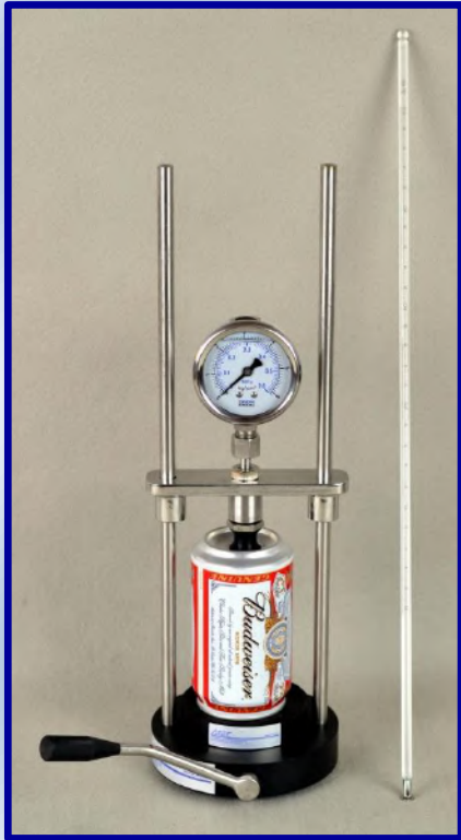
CO 2 EASY with analog pressure indicator & thermometer
