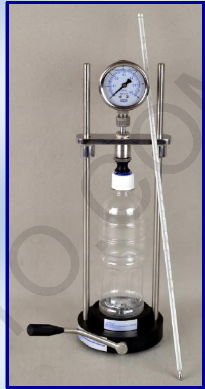
CO 2 EASY with analog pressure indicator & thermometer
