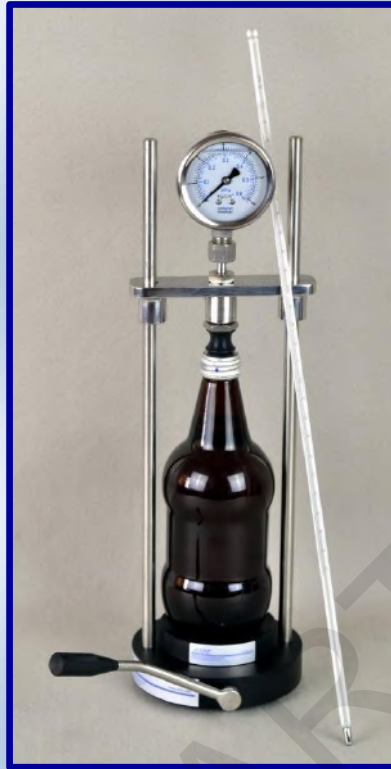
CO 2 EASY with analog pressure indicator & thermometer
